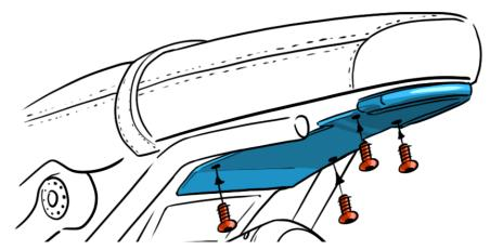
**EN**\_ After removing the original license plate holder, fix the Tail Tidy plate with four screws supplied in the kit as shown in the drawing.
