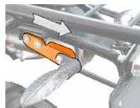
Reposition the indicators using the brackets code 1640.
