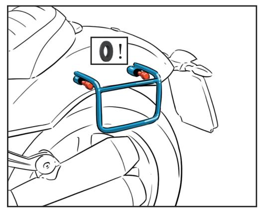
**EN**\_Remove the original screws, taking care not to drop the original plastic spacers from the fender, as **they must be reused**. Position the frame and secure it using the original screws.
