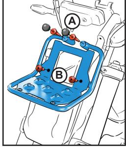
EN Remove the original screws indicated by the arrows. Position the luggage rack and secure it at point A with the long screws and at point B with the short screws provided in the kit.
